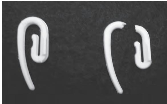
The student thinks that it is odd that the material the hooks are made from is referred to as plastic when the hooks don't show plastic behaviour.
