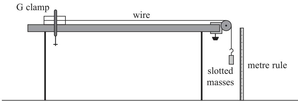
Masses were added up to a maximum of 3.30 kg. Each time a mass was added the extension of the wire was calculated.
